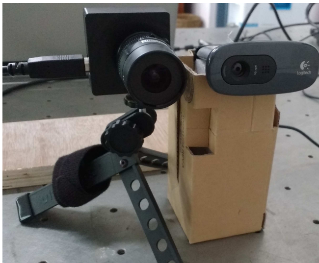
Figure 4.1: Set-up for DVS gesture recording
